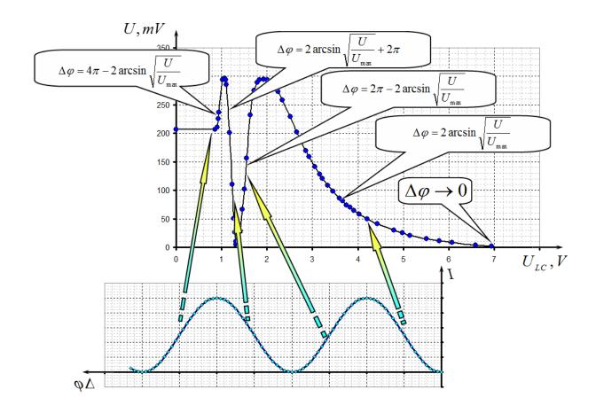
Results of calculation of  $(\Delta \varphi)' = \arcsin \sqrt{\frac{U}{U_{max}}}$  and correct values of phase shift  $\Delta \varphi$  are shown in the figure below.
