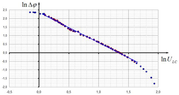
It can be seen from the graph that in the range of 1 V to 5 V the function is almost linear, which justifies the applicability of the power law. The power in that equation is equal to the slope of the graph, its numerical value is  $\beta \approx 1.75$ .
