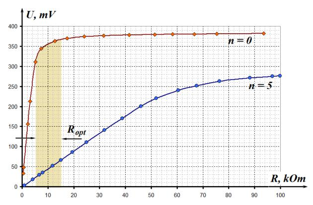
2.1.3 In table 2 the results are shown of the measurements for the voltage as a function of the number of light filters at different values of resistance.
