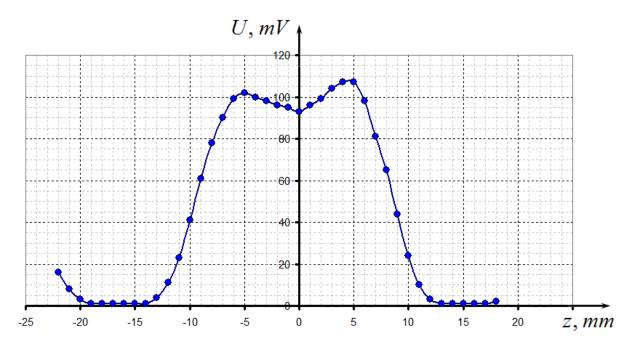
2.4.2 The shape of the curve indicates that  $\Delta \varphi_0$  lies at the ascending part of the relation between the intensity and the phase shift, which can be calculated as
