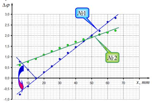
2.2.4 If two rulers are stacked together, then phase shifts simply add, and, theoretically, the intensity as function of phase shifts can be written as
