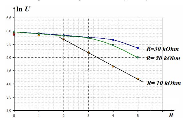
According to the graph above, by decreasing the resistance the dependence turns a linear function and further measurements should be made at the lowest resistance among given values, i.e. at  $R = 10 \, kOhm$ .
